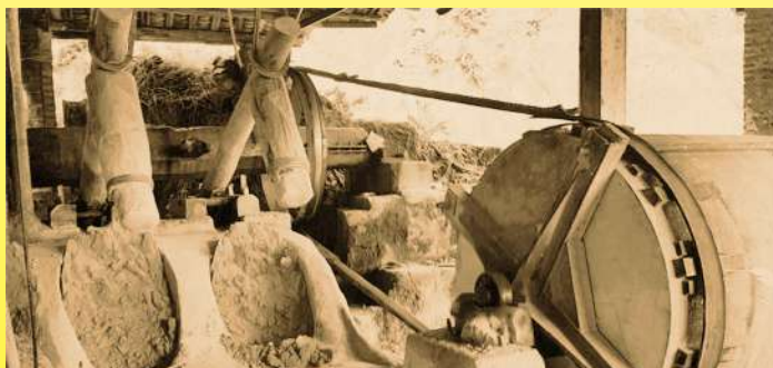
Traditional production machines ((水碓 shui duì) for production of powders used to make electric porcelain (private collection)
