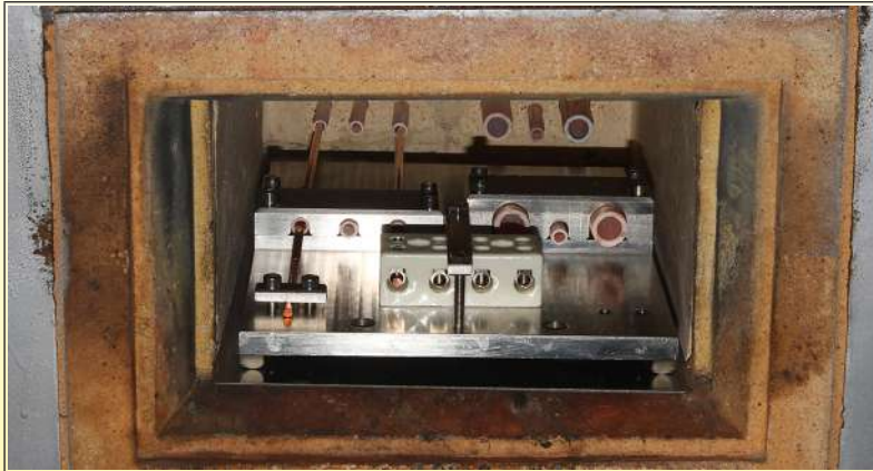
Test oven for the resistivity of ceramics as a function of temperature (Ultimheat Laboratory)
